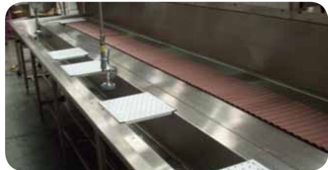
Trough bridges and obstruction-free pre-rinse sprays
